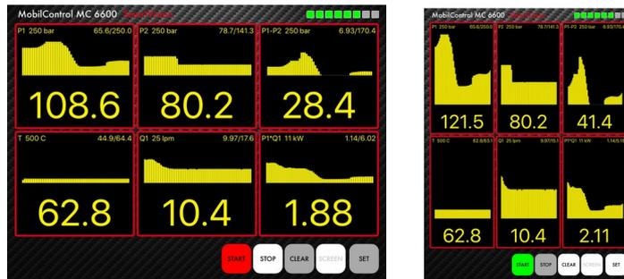
Current numeric reading, Min/Max reading with graphical representation of the recent 60 seconds.
